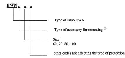
(a) IX... - wall box with bracket type or eyebolt type
