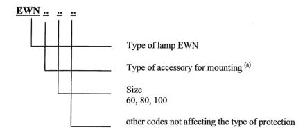
(a) T: suspension box with one entry X: suspension box with 4 entries GC: suspension box with eyebolt IX: wall box with 30 ° bracket
